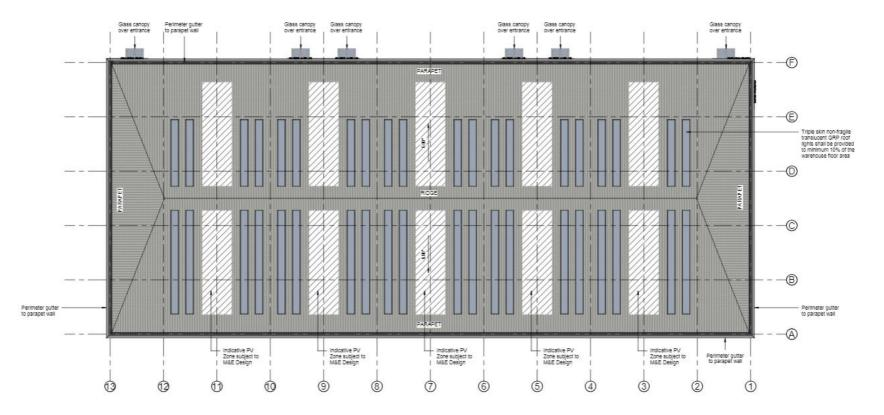
Proposed Roof Plan Scale @ 1:200
